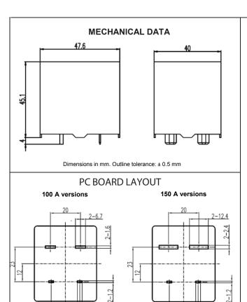
Dimensions in mm. Tolerance: ± 0.1 mm
