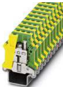
Ground modular terminal block, Connection method: Screw connection, Cross section: 2.5 mm 2 - 25 mm 2 , AWG 12 - 4, Width: 12.2 mm, Color: green-yellow, Mounting type: NS 35/15-2,3
