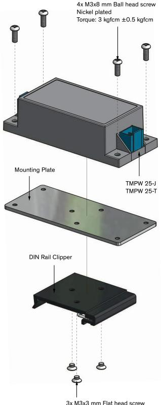
3x M3x3 mm Flat head screw Nickel plated
