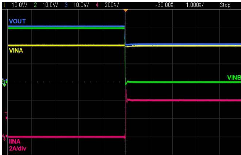
Figure 3. Diode-OR Using Figure 2. VINB's Voltage Drops Out, VOUT Settles to VINA, which Carries the Load
