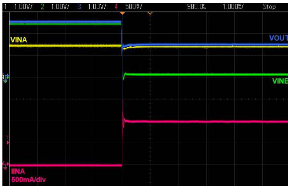
Figure 6. Low Voltage, Diode-OR Using Figure 5. VINB's Voltage Drops Out, VOUT Settles to VINA, Which Carries the Load
