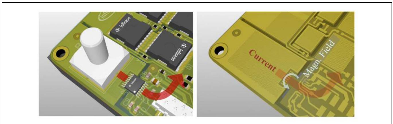
Figure 13 Hall sensor placement above current rail in middle layer
