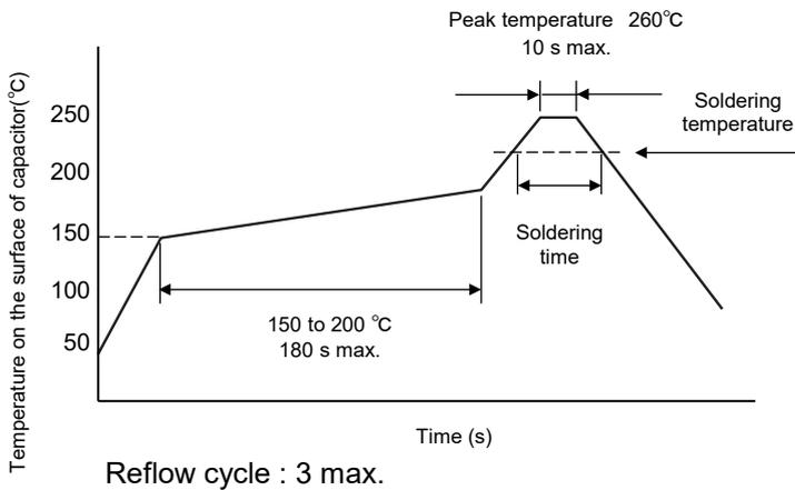
Soldering temperature and soldering time
