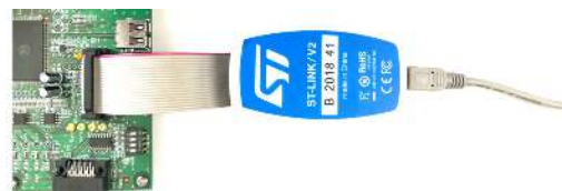
Figure 7. Debugger Connected with CN103
