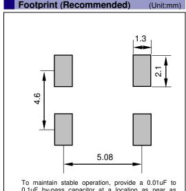
0.1uF by-pass capacitor at a location as near as possible to the power source terminal of the crystal product (between Vcc - GND).
