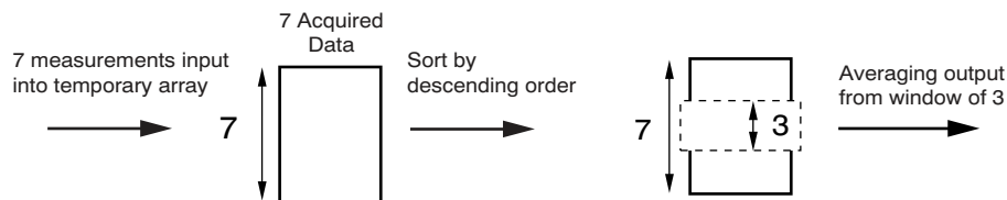
Figure 29. MAV Filter Operation (Patent Pending)
