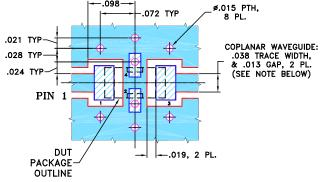
NOTES: 1. COPLANAR WAVEGUIDE PARAMETERS ARE SHOWN FOR ROGERS R04350B WITH THICKNESS .020"  $\pm$  .0015". COPPER: 1/2 OZ. EACH SIDE.
