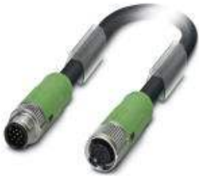
Sensor/Actuator cable, 17-position, PUR/PVC, black RAL 9005, shielded, Plug straight M12 SPEEDCON, A-coded, on Socket straight M12 SPEEDCON, A-coded, Cable length: 3 m
