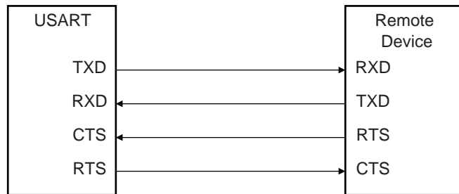
Figure 105. Connection with a Remote Device for Hardware Handshaking
