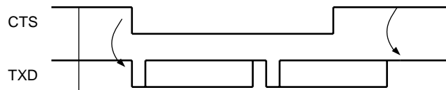
Figure 107. Transmitter Behavior when Operating with Hardware Handshaking
