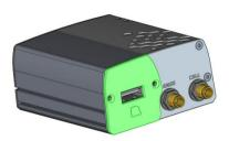
Place the replacement cover-plate (supplied with the IoT card) over the end of the connector on the IoT card and line up the two screw holes.
