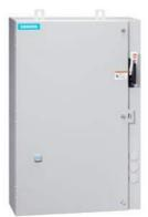
Non-reversing motor starter Size 0 Three phase full voltage Solid-state overload relay OLRelay amp range 0.75-3.4A 110-120/220-240VAC 60HZ coil Combination type 3Amp circuit breaker Encl NEMA type 4X 304 S-steel Water/dust tight noncorrosive Extra-wide enclosure
