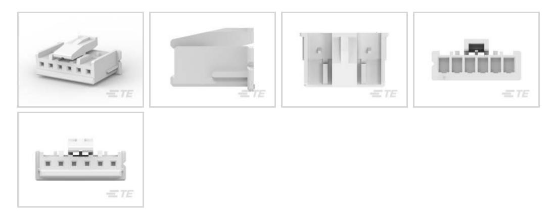
Connector Product Type: Housing Connector & Housing Type: Receptacle Connector System: Wire-to-Board Number of Positions: 6 Centerline (Pitch): 2.5 mm [.098 in ]
