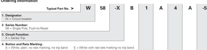
B = White with red rate marking, red trip band F = White with black rate marking, no trip band C = White with black rate marking, red trip band K = Black, plain, no rate marking, no trip band
