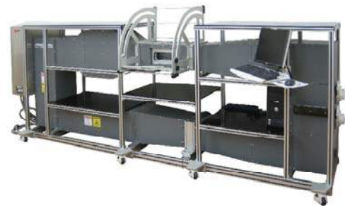
Fig. E: FDK Original Wind Tunnel
