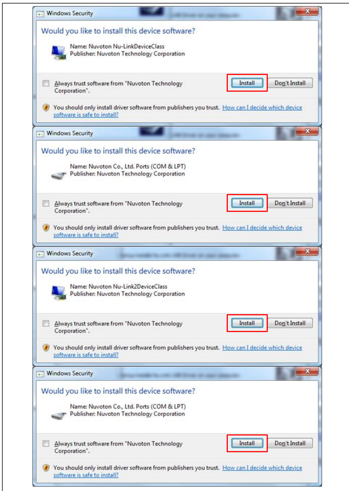
Figure 4-2 Nu-Link USB Driver Installation
