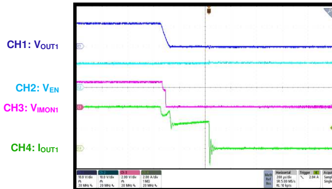
Current Limit 12V e-fuse, I_{OUT} increases slowly
