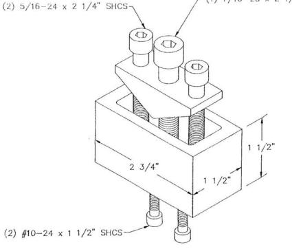
NOTE: A template can be made to these dimensions; or the 3 screw holes can be drilled (as per the instruction sheet) on these centers.
