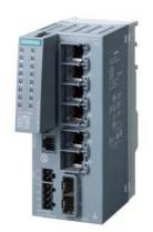
SCALANCE XC206-2SFP G EEC manageable Layer 2 IE switch; IEC 62443-4-2 certified; 6x 10/100/1000 Mbit/s RJ45 ports; 2x 1000 Mbit/s SFP; 1x console port; diagnostics LED; redundant power supply; with painted printed-circuit boards; NAMUR NE21-compliant; temperature range -40 °C to +70 °C; assembly: DIN rail/S7 mounting rail/wall; redundancy functions; office features (RSTP, VLAN,...); PROFINET IO device; Ethernet/IP-compliant; C-PLUG slot;
