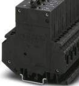
Thermomagnetic circuit breaker, 1-pos., normal blow, 1 N/C contact, with universal foot for mounting on NS 32 or NS 35
