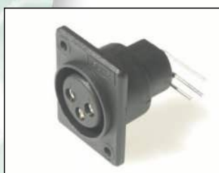
XACFR / PC 3 Pin horizontal lateral right PCB mounting Female XLR with self-tap screw fixing. Vertical PCB mounting versions ACF / PCS and XACF / PCS available. Nickel Silver plated Brass contacts. ACFR / PC (CP30016) XACFR / PC (CP30017) ACF / PCS (CP300125) XACF / PCS (CP30014)
