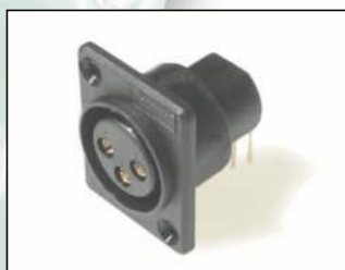
ACF / PC 3 Pin right angle PCB mounting Female XLR with counter sunk mounting holes for M3 screw fixing. XACF / PC has non counter sunk mounting holes for self-tap screw fixing. Nickel Silver plated Brass contacts. ACF-PC (CP30015) XACF-PC (CP300151)
