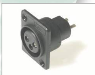
ACF 3 Pin chassis mounting Female XLR with counter sunk mounting holes for M3 screw fixing. XACF has non counter sunk mounting holes for self-tap screw fixing. Nickel Silver plated Brass contacts. ACF (CP3001) XACF (CP30012)
