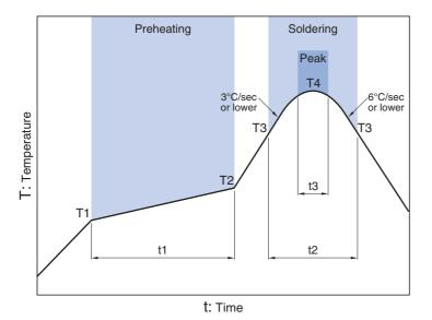
Soldering Preheating Critical zone (T3 to T4) Peak Temp. Time Temp. Time Temp. Time T1 T2 **T**4 t3\* t1 ТЗ t2 150°C 200°C 60 to 120sec 217°C 60 to 120sec 240 to 260°C 30sec max.
