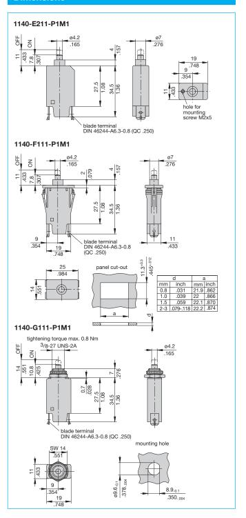
All dimensions without tolerances are for reference only. In the interest of improved design, performance and cost effectiveness the right to make changes in these specifications without notice is reserved. Product markings may not be exactly as the ordering codes. Errors and omissions excepted.
