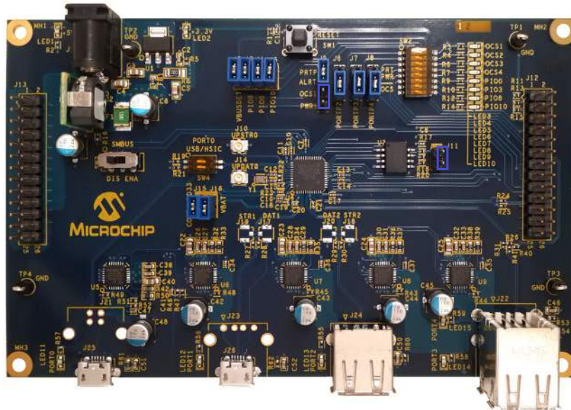
FIGURE 3-4: USB4604-1090 JUMPER CONFIGURATION
