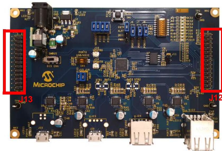
FIGURE 2-8: SYSTEM ACCESS HEADERS
