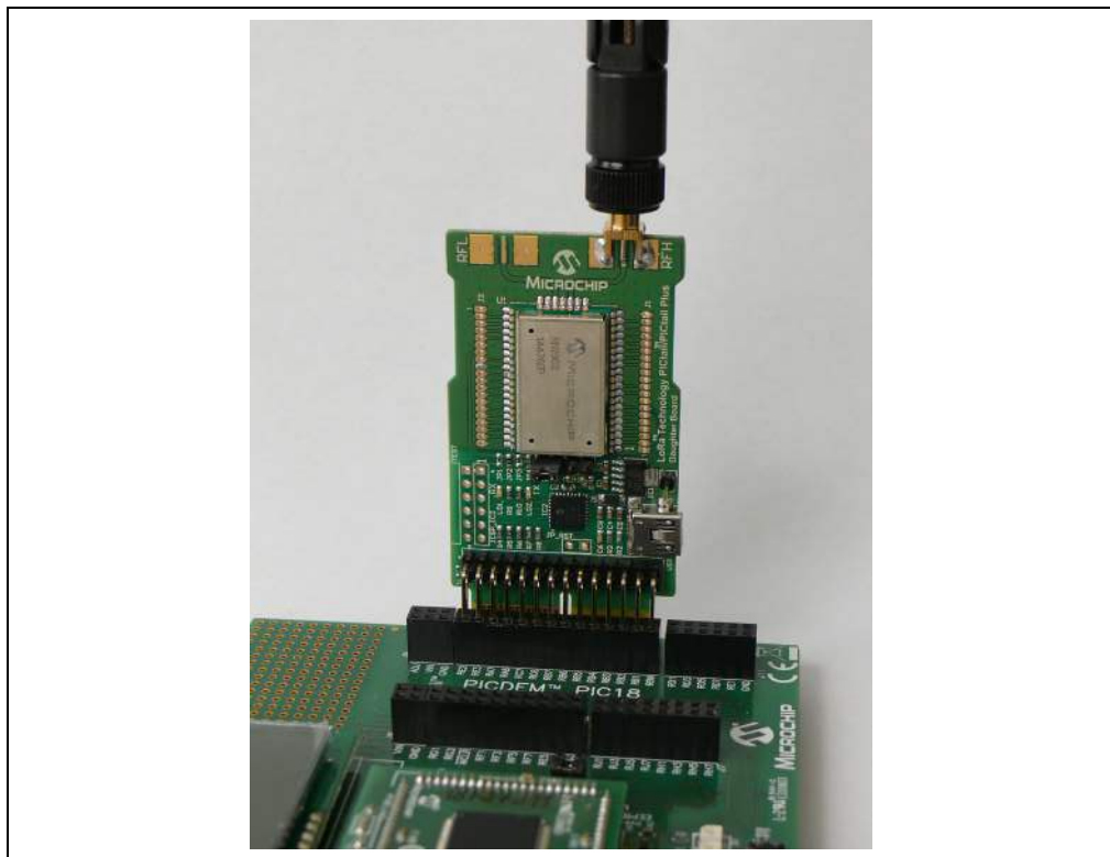
FIGURE 1-4: RN2903 LoRa™ TECHNOLOGY PICtail™/PICtail PLUS DAUGHTER BOARD CONNECTED TO PICDEM™ PIC18 EXPLORER DEMONSTRATION BOARD
