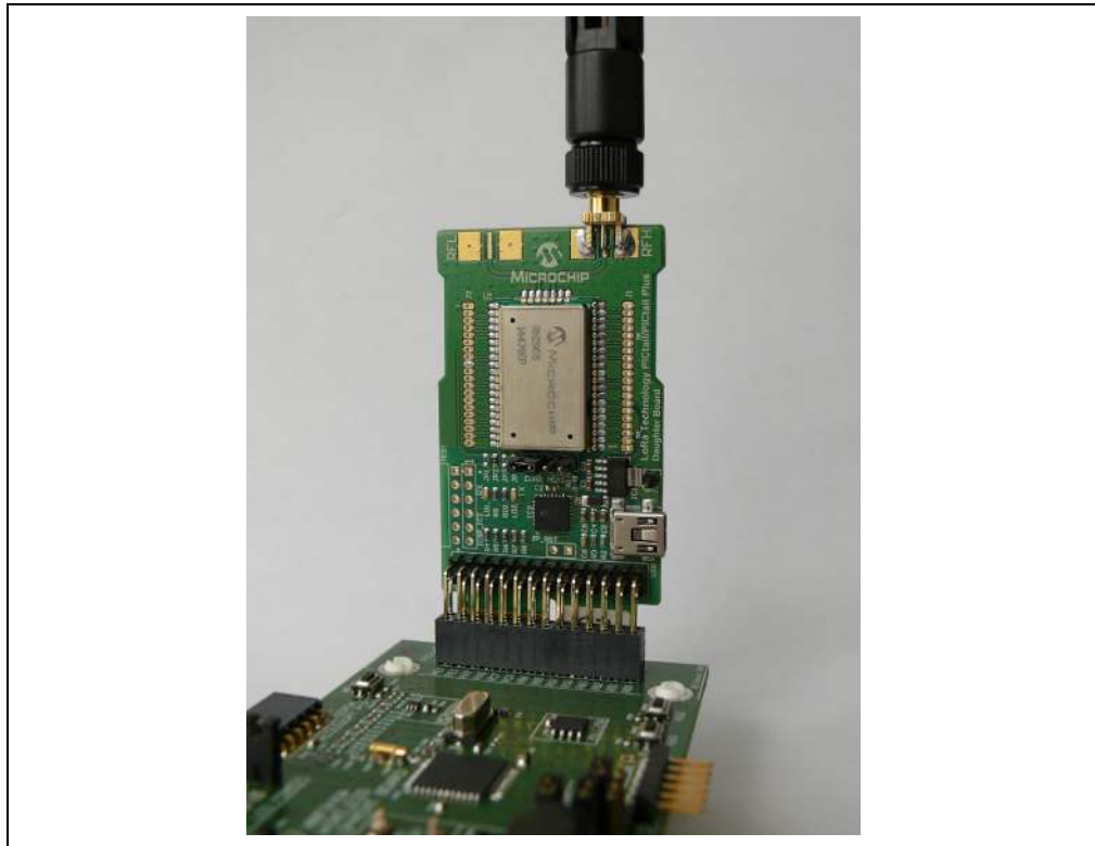
FIGURE 1-4: RN2903 LoRa™ TECHNOLOGY PICtail™/PICtail PLUS DAUGHTER BOARD CONNECTED TO PICDEM™ PIC18 EXPLORER DEMONSTRATION BOARD
