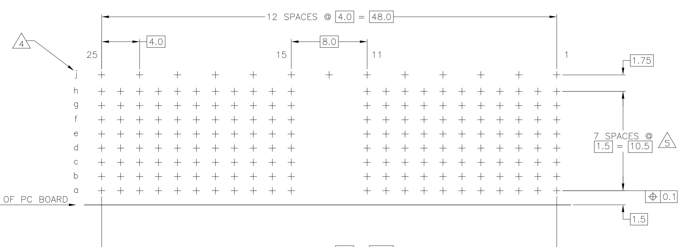
PLATED THRU HOLES PARAMETERS
