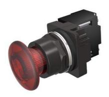
30mm BlackMax, Epoxy Coated Corrosion Resistant Complete Metal Unit Illuminated Push-Pull Operator Full Voltage, 24V AC/DC LED Lamp Mushroom Head Cap Small 1 3/4" (44.5 mm) Plastic, Red 3 Position Pull-Momentary/Push-Maintained UL Listed, CSA Certified NEMA 1,3,3R,4,4X,12,13 & Automotive Standards
