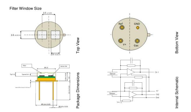
Note: Ensure that the sensor base is not in contact with the PCB in order to avoid shorts.
