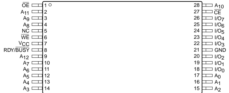
TSOP Package (8mm x 13.4mm) (H13)
