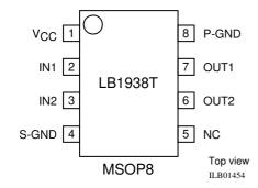
S-GND: GND for the control system P-GND: GND for the power system
