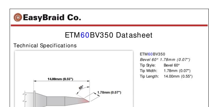
60 Type Cartridge1:325°C - 358°CRoHS Compliant2 / Lead Free:YESFor Use With:EB-5000S-1, EB-5000S-2
