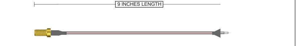
Connector A 132117RP SMA Jack Straight Brass Gold + Heatshrink 50 Ohm RG-316 Continuity/Hi-Pot Connector B FA1-NZSJ-C01-0 FAKRA Jack Straight Brass Nickel + Heatshrink
