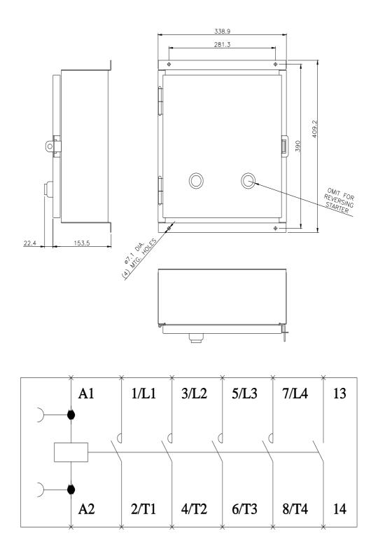
LEN00B004 Wiring Diagram
