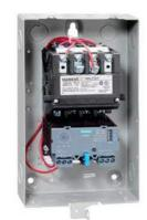
Non-reversing motor starter, Size 0, Three phase full voltage, Solid-state overload relay, OLR amp range 0.25-1A, 110V 50Hz / 120V 60Hz coil, Non-combination type, Enclosure type 12, Dust/drip proof for indoors, Standard width enclosure
