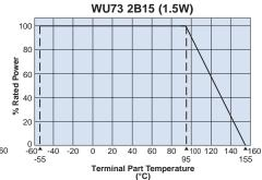
For resistors operated at a terminal part temperature of described for each size or above, the power rating shall be derated in accordance with the above derating curve.
