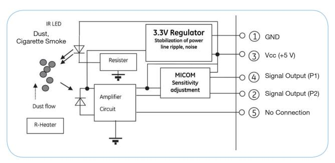
P1: small particle (1~ 2µm), P2: large particle (3~10µm)
