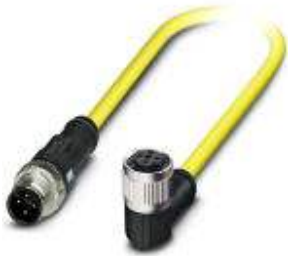
Sensor/Actuator cable, 4-position, TPE, yellow RAL 1021, Plug straight M12 SPEEDCON, A-coded, on Socket angled M12 SPEEDCON, A-coded, Cable length: 1.5 m
