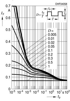
$I_{F} = f(t_{p})$ ; duty cycle D = parameter;  $T_{A} = 25^{\circ}C$
