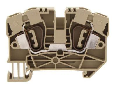
Ex feed-through terminal ATEX-certified, Tension-spring connection, Mounting type: Mounting rail TS 35/7.5, Rated cross-section: 6 mm², Width: 8.1 mm, Colour: Beige
