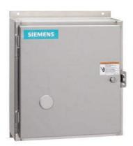
Non-reversing NEMA contactor, Size 4, Three phase full voltage, Contactor amp rating 135A, 3 wire (NO aux included), 208VAC 60Hz coil, Non-combination type, Encl NEMA type 4X 304 S-Steel, Water/dust tight noncorrosive, Extra-wide enclosure
