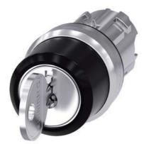
RONIS key-operated switch, 22 mm, round, metal, shiny, lock number 455, with 2 keys, 3 switch positions I-O-II, latching, actuating angle 2x45°, 10:30h/12h/13:30h, Key removal I+O+II, with laser labeling, upper case
