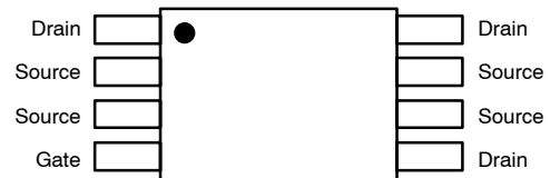
Figure 2. Pinouts for Single Die TSSOP
