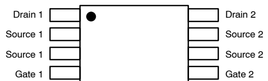
Figure 3. Pinouts for Dual-Die TSSOP
