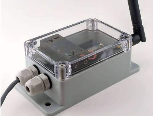
Pic. 20. 2xAAA battery holder applied to a transparent lid (assembled view)
