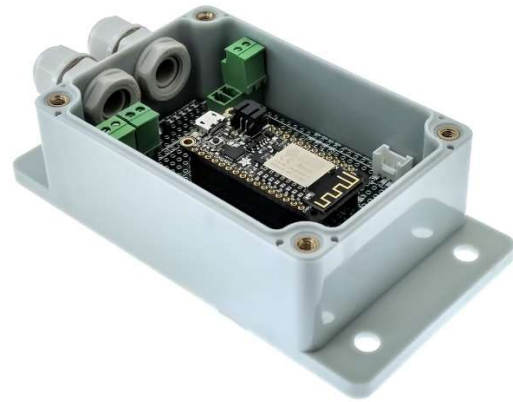
Pic.9. qBox Enclosure Plus Kit with Adafruit Feather Compatible (AFC) board installed
