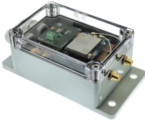
Pic. 24. LTE GPS BG96 tracker with RS485 port
