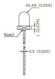
Units: mm / tolerance = +/-0.25mm unless otherwise specified
