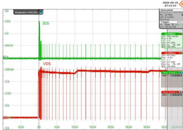
Figure 32 – Drain Voltage and Current Waveforms. 115 VAC, 0 mA Output. Upper: I_{DS} , 500 mA / div. Lower: V_{DS} , 40 V / div., 5 ms / div. I_{DS(MAX)} = 1.54\text{ A} , V_{DS(MAX)} = 171.1\text{ V} .
