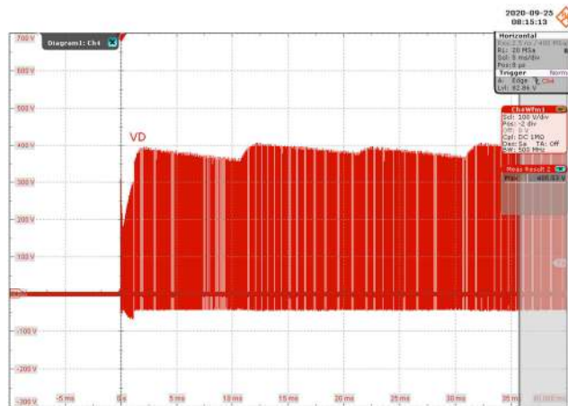
Figure 46 – Freewheeling Diode Voltage Waveforms. 115 VAC, 550 mA Output. 40 V / div., 5 ms / div. V_{MAX} : 174.9 V.
