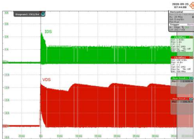
Figure 27 – Drain Voltage and Current Waveforms. 85 VAC, 550 mA Output. Upper: I_{DS} , 500 mA / div. Lower: V_{DS} , 40 V / div., 5 ms / div. I_{DS(MAX)} = 1.26 A, V_{DS(MAX)} = 123.6 V.
