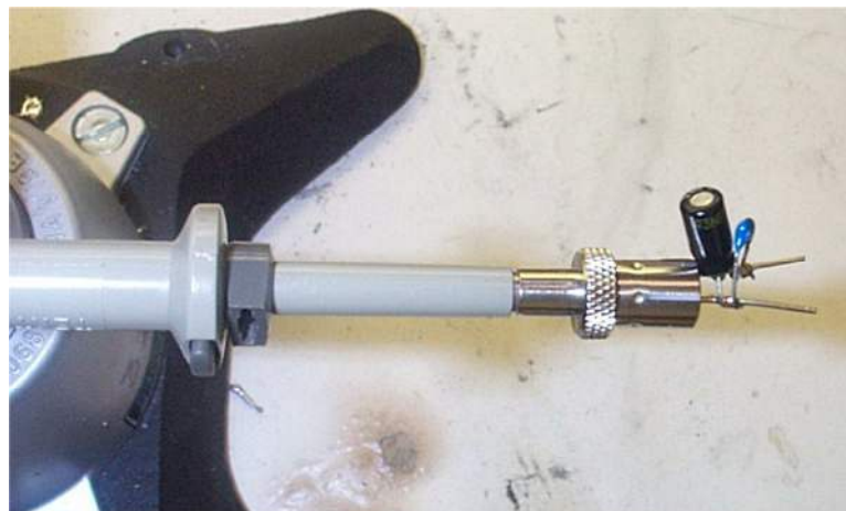
Figure 66 – Oscilloscope Probe with Probe Master ( www.probemaster.com ) 4987A BNC Adapter. (Modified with wires for ripple measurement, and two parallel decoupling capacitors added.)
