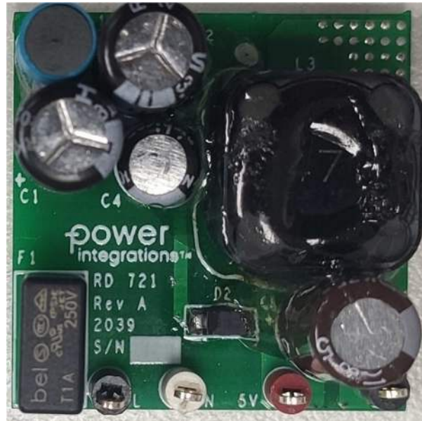
Figure 1 – Populated Circuit Board Photograph, Top.
