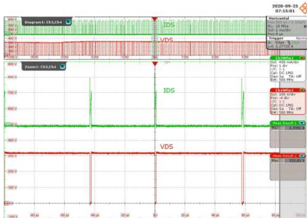
Figure 19 – Drain Voltage and Current Waveforms. 85 VAC, 550 mA Output. Upper: I_{DS} , 400 mA / div. Lower: V_{DS} , 40 V / div., 20 \mu s / div. I_{DS(MAX)} = 1.09 A, V_{DS(MAX)} = 126.8 V.
