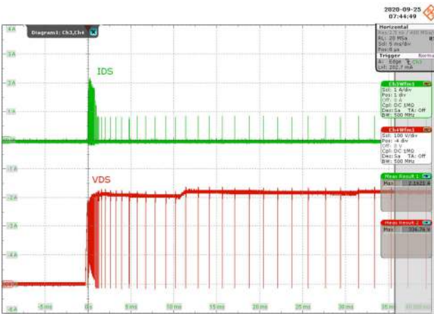
Figure 31 – Drain Voltage and Current Waveforms. 85 VAC, 0 mA Output. Upper: I_{DS} , 500 mA / div. Lower: V_{DS} , 40 V / div., 5 ms / div. I_{DS(MAX)} = 1.40\text{ A} , V_{DS(MAX)} = 126.8\text{ V} .
