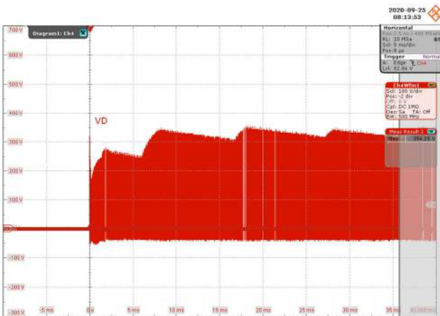
Figure 45 – Freewheeling Diode Voltage Waveforms. 85 VAC, 550 mA Output. 40 V / div., 5 ms / div. V_{MAX} : 130.6 V.
