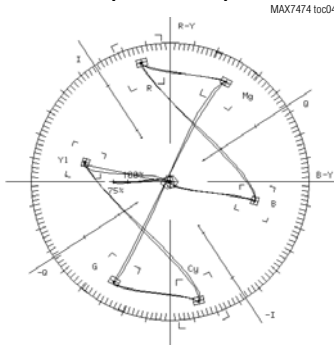
75% COLOR BAR VECTOR DIAGRAM (300m CABLE)
