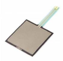
Attach the alligator clip extensions (regular alligator clip wires) onto the two metal prongs on the end of the Force Sensitive Resistor.
