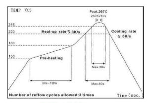
IR Reflow Soldering (1) Time of IR reflow soldering at maximum temperature point 260°C : 10s
